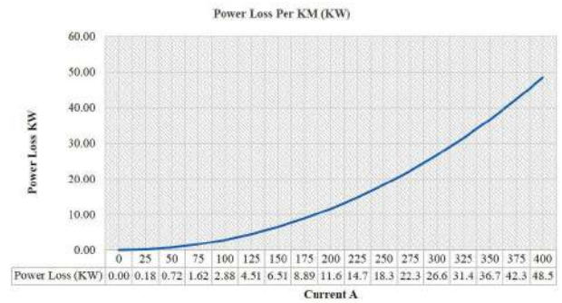
Figure 3 Power Loss per KW
