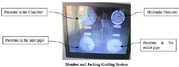
Figure 2: Operation monitoring from the control cabin
