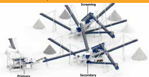
Complete Crusher Plant
